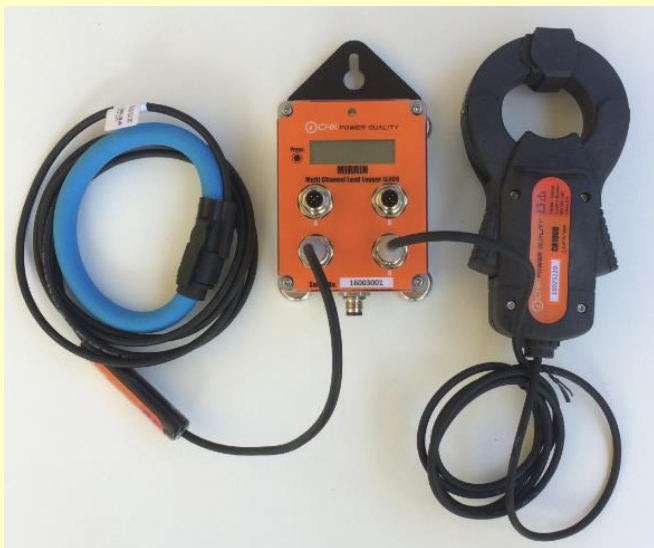
Figure 1: MLL (middle) with current sensor options - flexible current probe (left) and clamp-on current probe (right)
