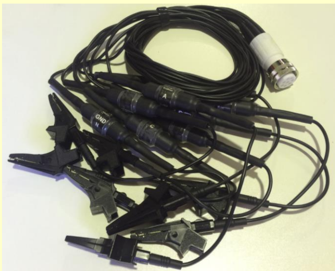
Figure 6: Fused three phase lead for MIRO PQ45 with banana plugs and detachable small clamps (crocodile clips); Part number: 1AVL8-B
