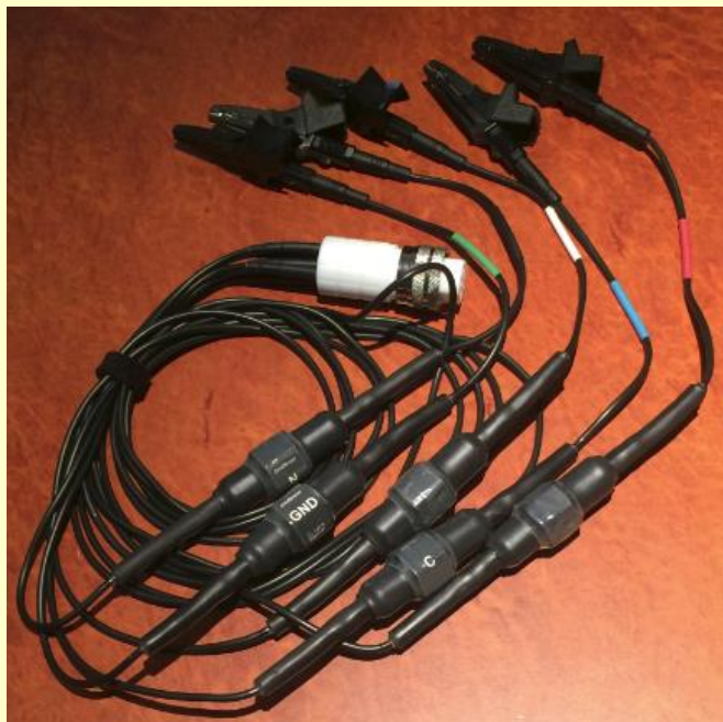
Figure 2: Fused three phase lead for MIRO P45, with banana plugs and detachable small clamps (crocodile clips); Part number: 1AVL5-B
