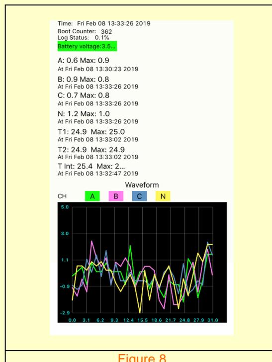
5. The user can also perform configuration changes via the Citrus Lite app to adjust measurement intervals and alarm settings.
