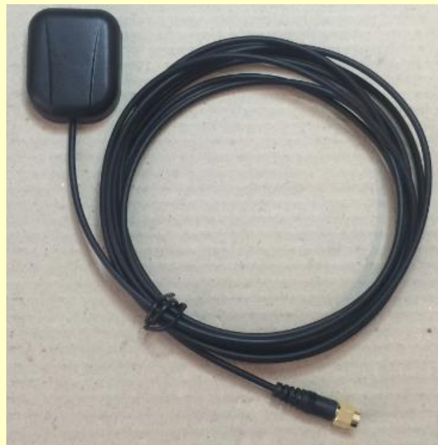
Figure 3: Active GPS antenna; Weight: 100g; Cable length: 3m; Operating voltage: (2.5-12) VDC current: (11-13) mA; Operating frequency: 1.575.42MHz Part number: 1AGPSANTM (magnetic mount)
