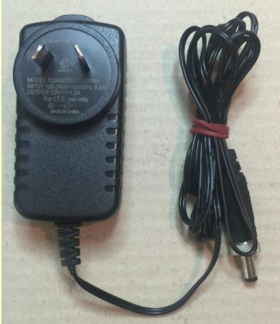
Figure 5: Regulated DC adaptor; Input voltage: (110-240) Vrms; Rated output: 12VDC at 1.5A; Weight: 150g; Cable length: 1.8m; Part number: 1ADC12VPS
