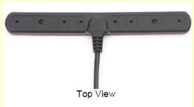
Figure 4: T-bar penta-band cellular antenna Cellular technologies: GSM / CDMA / PCS / DCS / UMTS / WCDMA; IP rating: IP67 (waterproof); Weight: 40g; Dimensions (L x W x H) mm: 105.7 x 14 x 6.5
