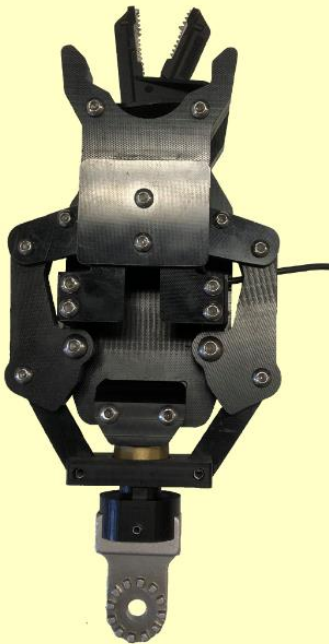
Figure 4: Current transformer probe and voltage clamp installer with voltage clamp captured and jaws opened
