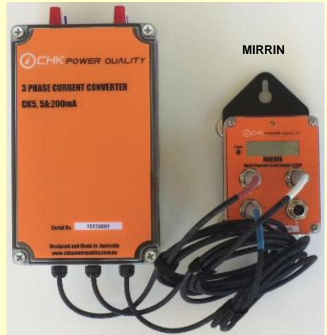
Figure 3: CK1/CK5 connection to the MIRRIN
